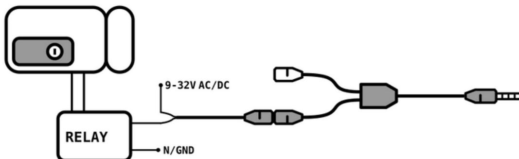
The input contact must be connected to the open/close sensor supplied and is necessary to detect the closed state of the automation. The open/close sensor must be applied to the automation in such a way that when the sensor is closed (plates approached) the automation is closed. Each position of the sensor other than the closed status position will consider the automation open.
