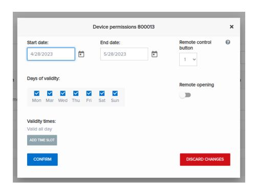
It is possible to set different permissions for each device. You can select a start date and an expiry date, the days of validity and the time slots in which you want to enable the user to open (for example it is possible to enable openings only from Monday to Friday, from 9am to 1pm and from 2pm to 6pm).
